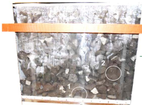
Picture of the set-up of the ITW-investigations. 1: area with big voids. 2: area with small void fraction
